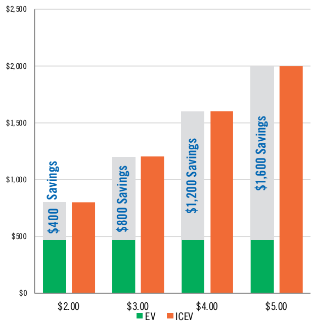
Figure B: Annual Fuel Costs to Power an EV vs. 30 MPG ICEV at Varying Gasoline Prices (assume 12,000 miles/year) 22
